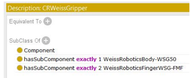
Fig. 6. View of the Protégé editor showing the sub component axioms of a particular pinch gripper class called CRWeissGripper
