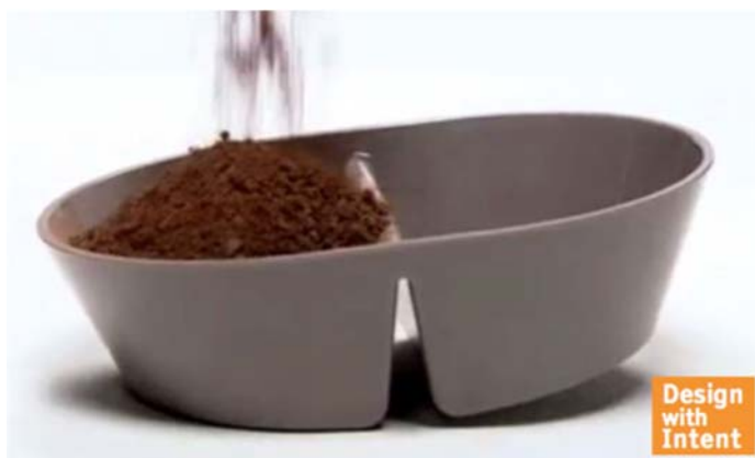
Figure 24 Example for feedback through form. Royal VKB's 100g/250g Balancing Bowls are weighted so they tilt noticeably and audibly when the 'portion size' is reached when filling. Adapted from Lockton, 2011.
