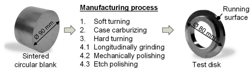
Figure 2. Manufacturing process of sintered test disks.
