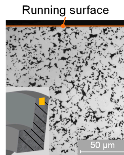
Figure 6. Light microscope picture of bulk porosity of a sintered disk sample for the twin-disk test rig.
