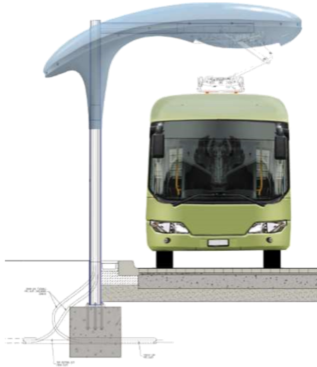
Figure 2.3: Charging electric bus via an overhead pantograph [33]
