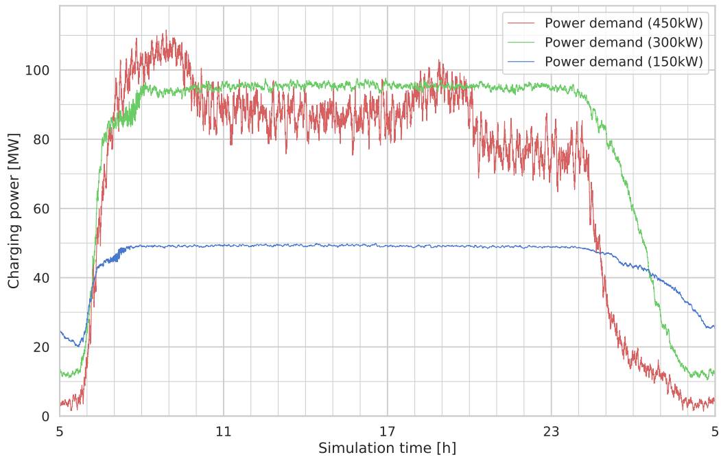
Figure A.9: Instantaneous aggregated charging power demand for 450, 300, and 150 kW during day 5 operations with same chargers count (333 chargers for all cases).
