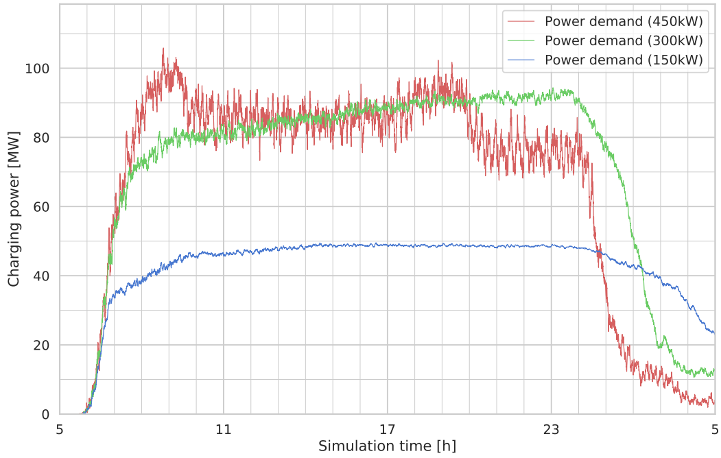
Figure A.8: Instantaneous aggregated charging power demand for 450, 300, and 150 kW during day 1 operations with same chargers count (333 chargers for all cases).
