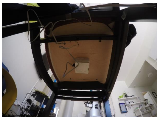
Figure 15 Motion sensor under the test subjects' chair, see the white box (image: author, 09/06/15)
