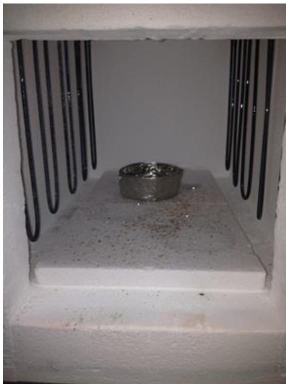
Figure 18. Photograph showing the platinum crucible holding the infiltrated template after placement in the oven for calcination.
