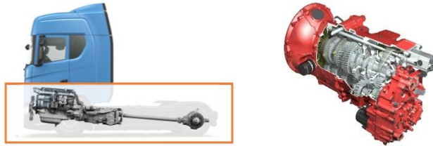
Figure 2. An illustration of a Scania truck powertrain (left), with a heavy-duty gearbox (right)
