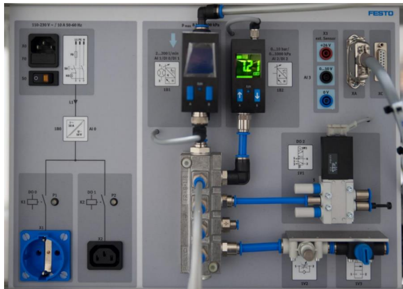
Fig. 9. Energy monitoring hardware of the xPPU
