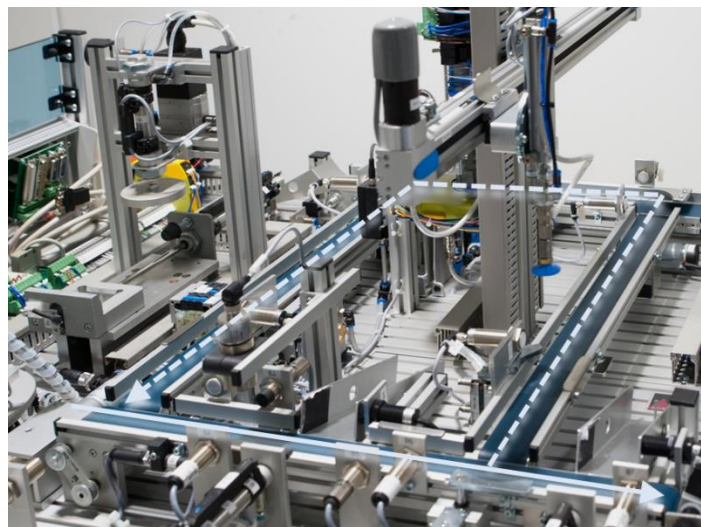
Fig. 6. Conveyor System of the xPPU
