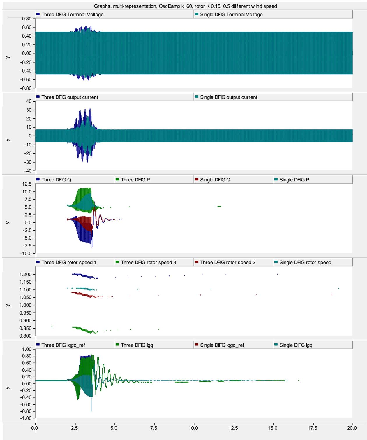
Fig. 2-55 SSR mitigation by damping controller with a three-DFIG system and single DFIG system (from top to bottom: DFIG terminal voltage, DFIG output current, DFIG output reactive power and active power, DFIG rotor speed, DFIG reactive current from grid-side converter)
