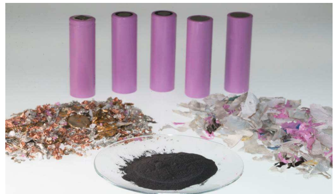
Fig. 9. Recycled material fractions from electrohydraulic fragmentation process: metals (left), black mass (front), plastics (right).
