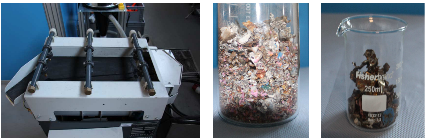
Fig. 5. Wet separation table (left). Exhibits of coarse fraction (mid), battery housings (right) after fragmentation and separation.
