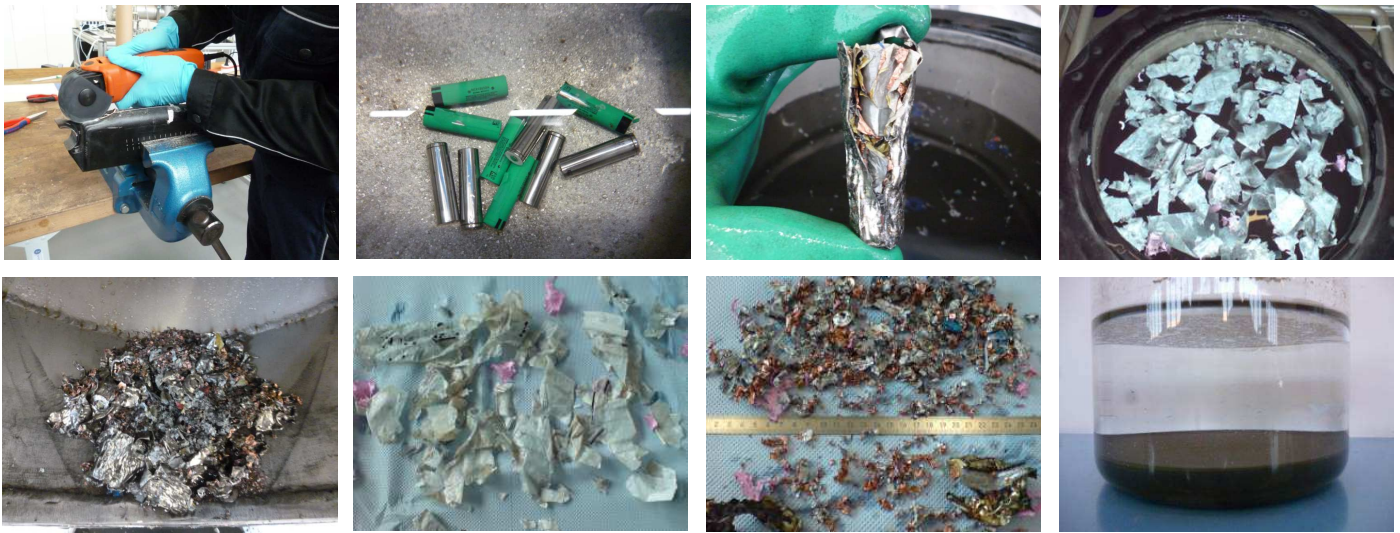
Fig. 4. Processing of batteries including manual dismantling, electrohydraulic fragmentation, segregation with sieving methods and purification.
