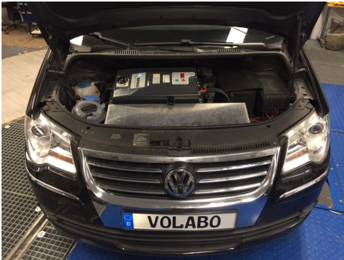
Fig. 7. First part of the battery pack behind the radiator grill and on board charger in the upper part of the motor compartment.
