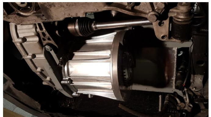
Fig. 6. Gearbox with constant ratio (left) and electrical machine (right) in the lower motor compartment.
