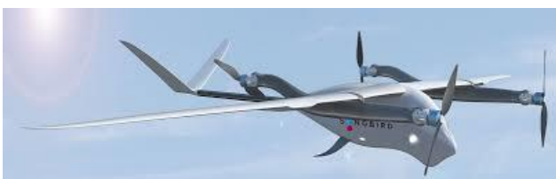
Fig. 1. ‘Tilt Rotor’ Configuration in Cruise ©Germandrones
