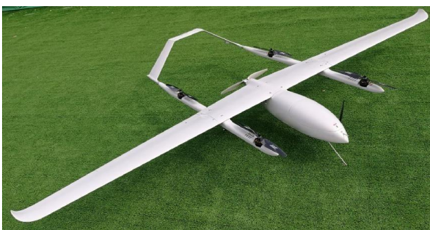
Fig. 2. ‘Hover Plus Cruise’ Configuration ©Icarus Drone Services
