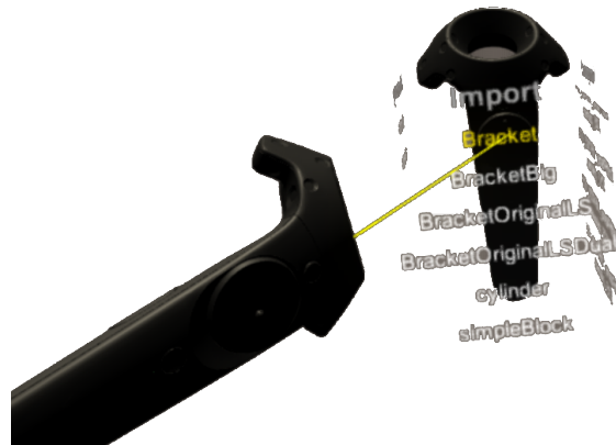
Figure 5.2.: The menu – The user can scroll sideways through different columns like Import , Create or Boolean using the trackpad. By selecting a menu entry with the other controller the corresponding command is executed.
