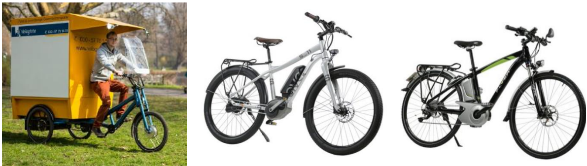
Figure 1: Different HEHV types: A three-wheeled cargo-bike (left), a Pedelec (middle) and a S-Pedelec (right) (ExtraEnergy e.V., 2014)
