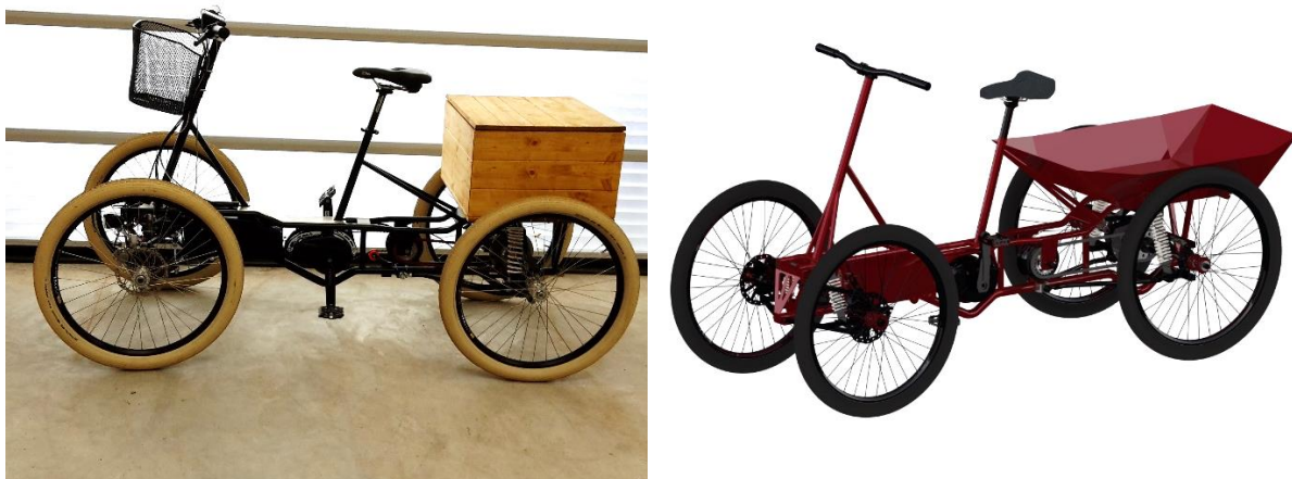
Figure 3: QuadRad prototype (left) and mechanical design (right). The QuadRad has four wheels and is equipped with a mid-mounted motor. It fulfills the legal requirements for pedelecs and therefore is categorized as a bicycle.
