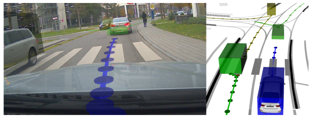
Fig. 7. Forward simulation of belief to generate multi-agent trajectories.
