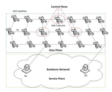
Fig. 1. Proposed SDN-enabled LEO constellation architecture.
