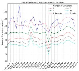
Fig. 5. Optimal average flow setup time ms for various simulation GMT hours as a function of the number of controllers K. Furthermore the average flow setup time is illustrated for the static approach with blue dotted line for K-6
