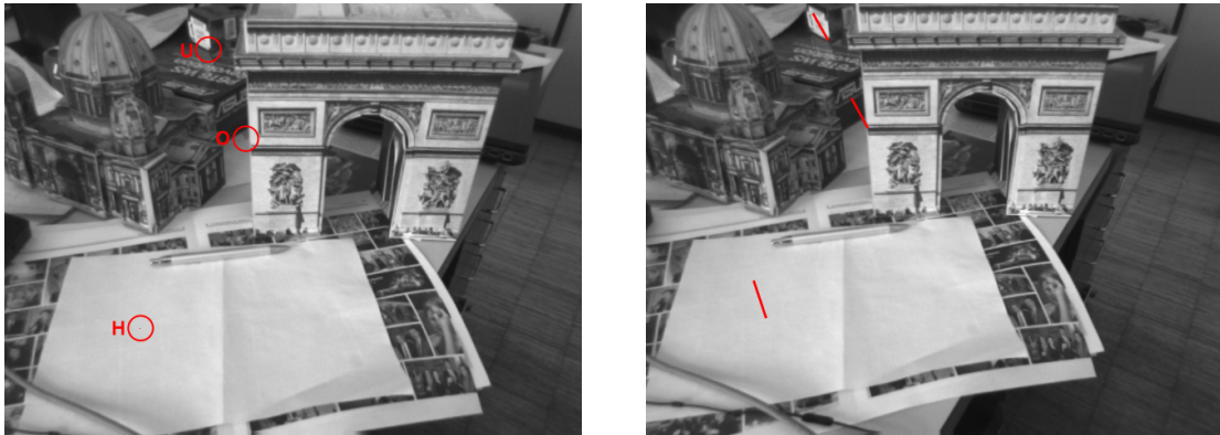
(a) Reference image with selected points: unique (U), homogeneous (H), occluded (O). (b) Second matching image with search space along epipolar lines.
