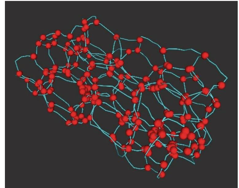
Topology of a metallic foam, extracted by image processing from tomography data (figure from DFG-ANR-application)
