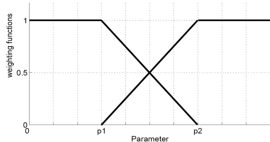
Example of two weighting functions  $\omega_1(p), \omega_2(p)$
