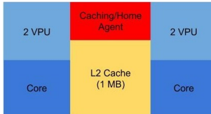
Figure 10: Diagram demonstrating an overview of a tile in KNL Architecture.
