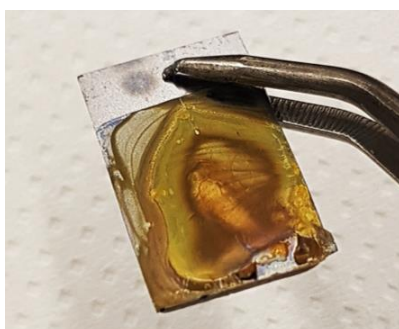
Figure 2.57. Photo of a P thin film on a Si substrate, prepared using a K 3 P 7 / en solution.
