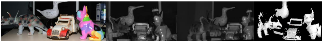
Figure 5.9: Collecting dataset of 4 additional toy objects. (from left to right) : RGB images of objects given to aid perception; the actual stereo images acquired by the scanner; triangulation of the stereo capture.
