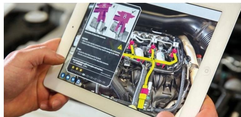
Note. Still of Re'flekt One and Bosch's Common Augmented Reality Platform (CAP). The still exemplifies how information can be provided to car mechanics in a visual and intuitive way. Source. Bosch Auto Parts (2017).
