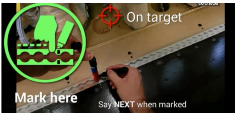
Note. Still of Accenture's AR system for the assembly of cabin seats in the Airbus 330. The still exemplifies the interactive work process in Augmented Assembly. Source. Accenture (2017).
