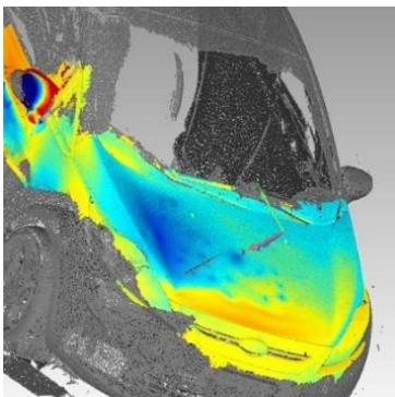
Note. Ngrain uses Voxels to assess collision, hail or scratch damage. The illustration exemplifies how AR can support the appraisal of damages. Source. Smith (2016).
