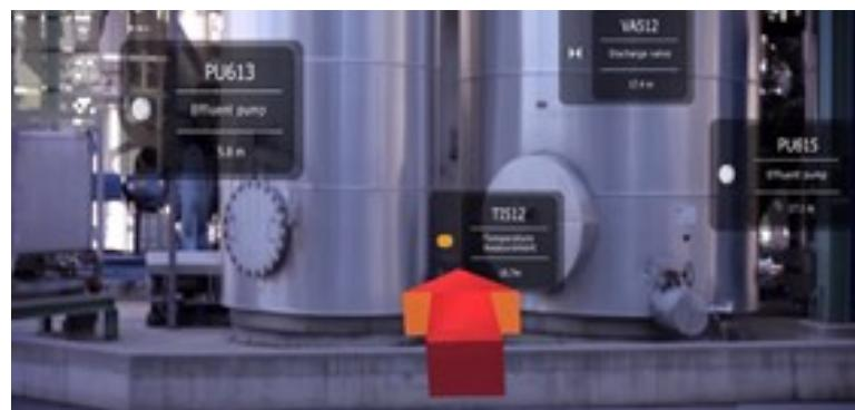
Note. Still of UBIK platform created by Augmensys. The still exemplifies how service technicians receive information in complex plant environments. Source. Augmensys (2014).
