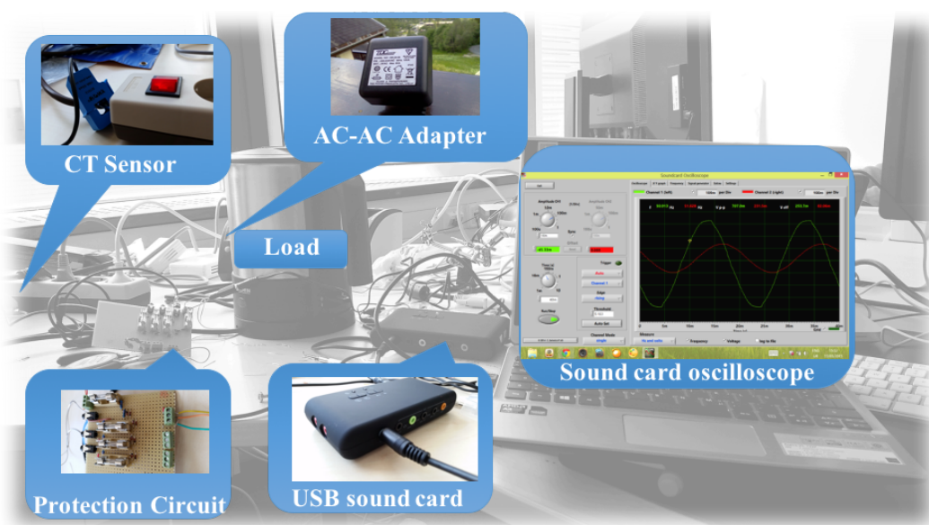
Figure 5.1.3: Sound card energy meter (line input)
