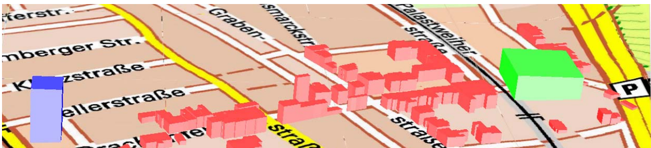
Fig. 7: A city model aspect was defined to show the combination of alternatives of different plannings. Here the tall version of the “blue” planning and the broad version of the “green” planning have been combined. A city model aspect is a multiparent workspace whose parents are the workspaces associated to the planning alternatives (cf. fig. 3).
