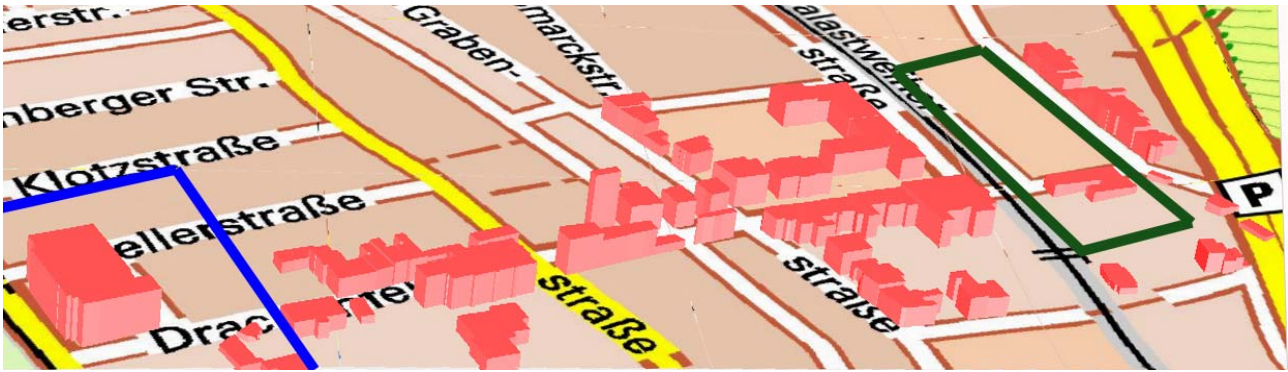
Fig. 4: Portion of a 3D city model. Two planning regions are described by their spatial extent: one on the left (blue) and another on the right (dark green). Each planning may comprise several competing alternatives as versions. Each alternative is assigned to one workspace which stands for a virtual copy of the 3D city model.
