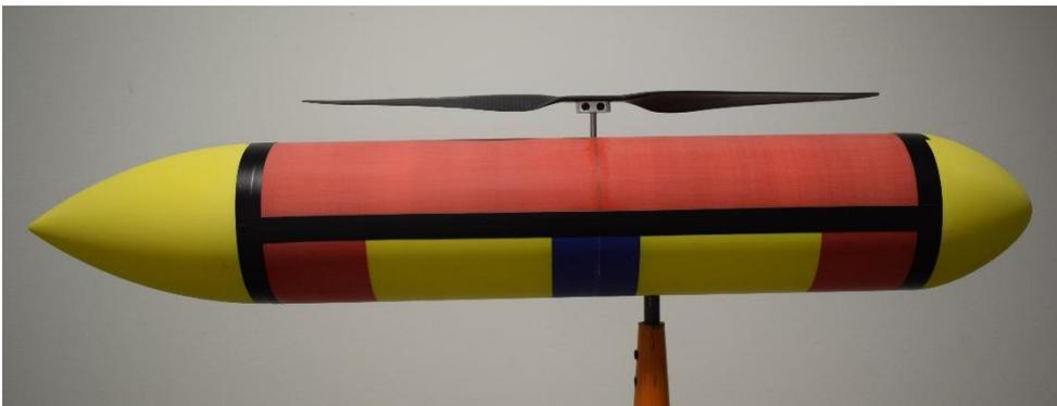
**Figure 3: Wind tunnel model in reference configuration (clean cylinder with rotor)**
