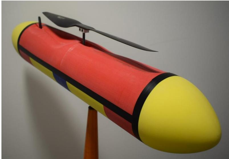
**Figure 2: Wind tunnel model with rotor recess and extended rotor and stop pin**
