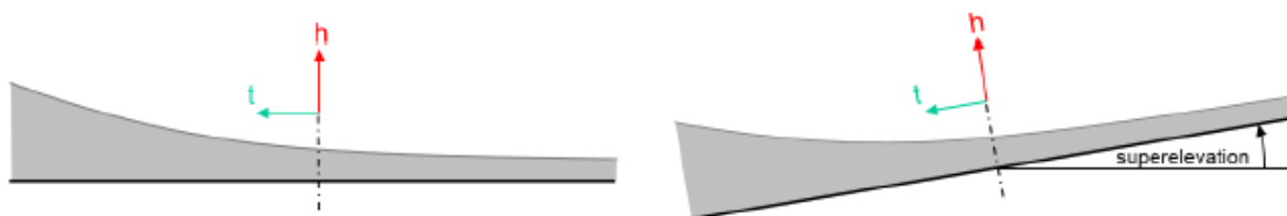
Abbildung 3.6 – Querprofile in OpenDRIVE [Dupuis et al., 2015, S.24]
