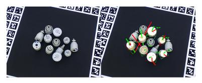
**Figure 5.25.** Pose and axis of ambiguity estimation on the T-LESS dataset. The green line represents the annotated ground truth axis, the red one is the estimated value.
