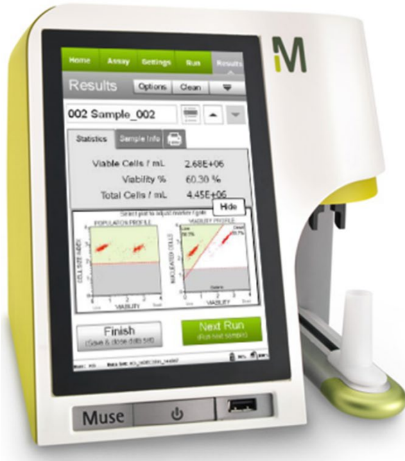
Fig. 4. Muse Cell Analyzer and cell viability assay. (A) The Muse Cell Analyzer from Millipore Merck is a small convenient device with only a footprint of 20 × 25 cm, a green excitation laser, and a multitude of pre-configured analysis options such as the viability assay. (B) With the use of the two dyes, one yellow non-membrane permeable DNA-binding dye and one red membrane permeable DNA-binding dye, live cells can be separated from dead and dying ones. (C) A plot is given of live and dead cells after analysis.
