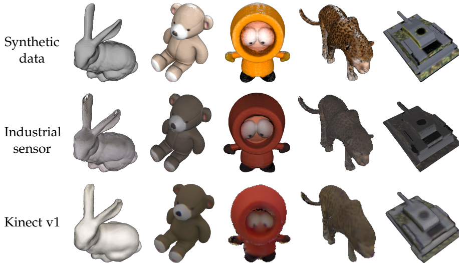
Figure 4.1: SDF-2-SDF reconstructions of the 3D-printed dataset objects captured with different RGB-D sensors. Colours vary due to difference between synthetic rendering and 3D-printed models, as well as camera radiometrics.
