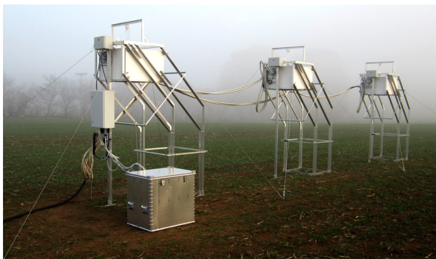
Figure 12: Greenhouse gas measurements using automated chambers
