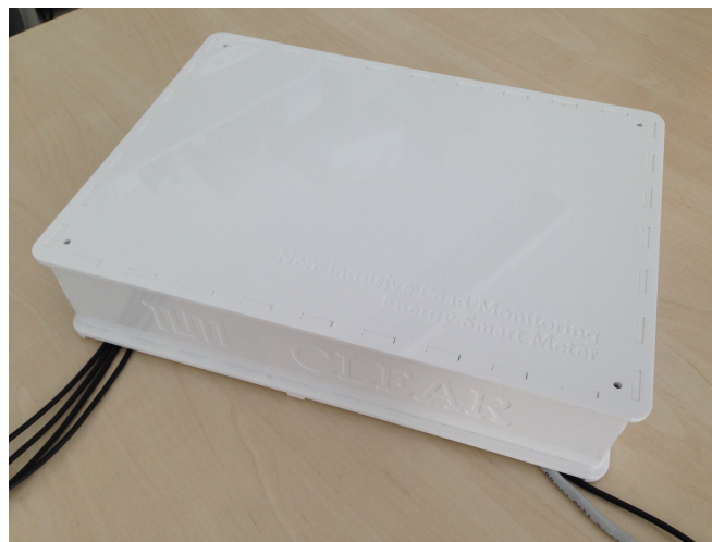
Figure 6.2.2: The data acquisition and processing component of the CLEAR system. The laser-cut acrylic enclosure contains three components: sensor board, DAQ board, and a Linux PC.
