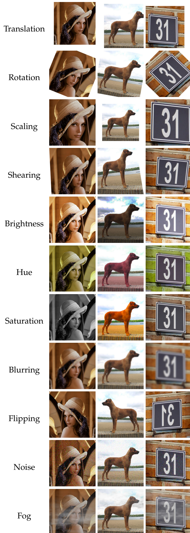
Figure 2.1: Examples for different types of data augmentation. Left: The "Lena" image [79], middle and right: examples from Imagenet and SVHN, respectively
