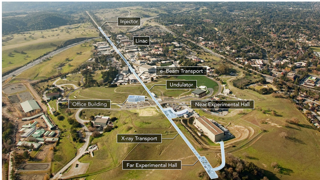
FIGURE 5.2: The aerial view of the SLAC area shows the major parts of the LCLS facility highlighted in blue. Taken from [194].
