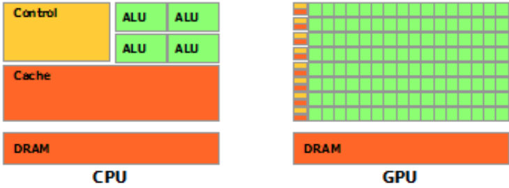
Figure 5.1.: Central Processing Unit (CPU) vs Graphical Processing Unit (GPU)[10](NOTE: Not to scale.)
