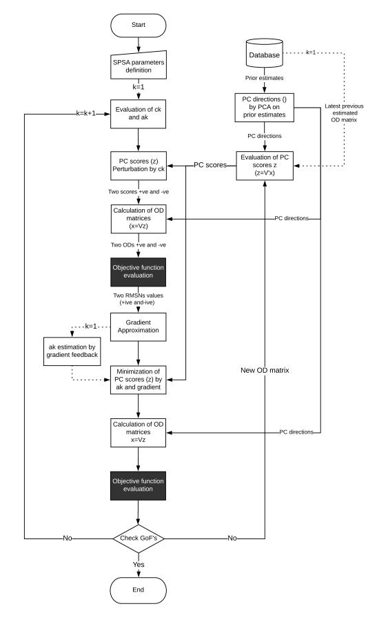
Figure 3.4: PC-SPSA algorithm flow chart
