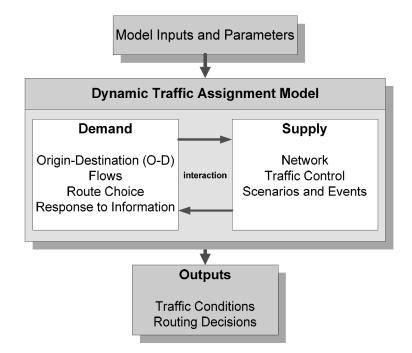
Figure 2.4: Generic interactions in a DTA model-(TRB, 2011)
