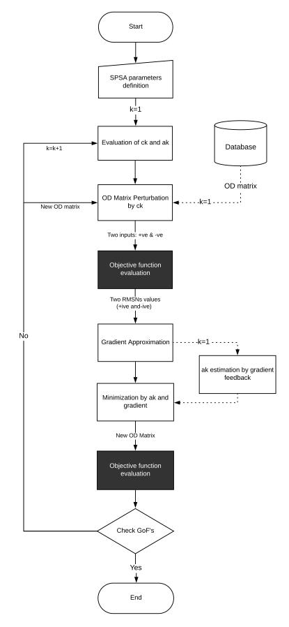
Figure 3.3: SPSA algorithm flow chart
