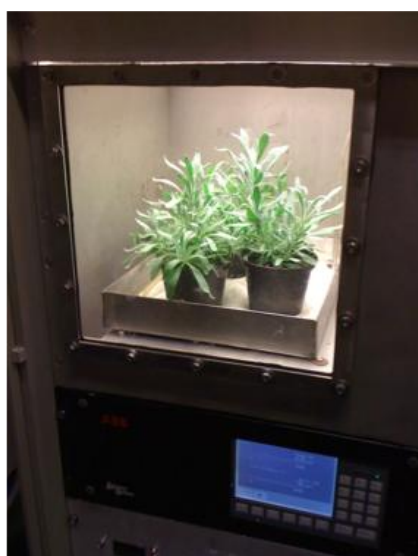
Figure 10. Gas chamber for incubation of plants with ^{13}\text{CO}_2 .
