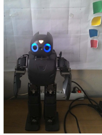
Fig. 3. The robot used in the study is a humanoid robot platform called Darwin-Op. The humanoid robot is expected to associate the presented colors to the desired predefined actions. The three colors to be associated to the actions are red, yellow and blue. The green color is used to indicate reward given when the action choice is the desired one.
