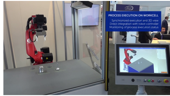
(b) Execution of the assembly task using a 6 DoF Comau Racer 7-14 robot.
