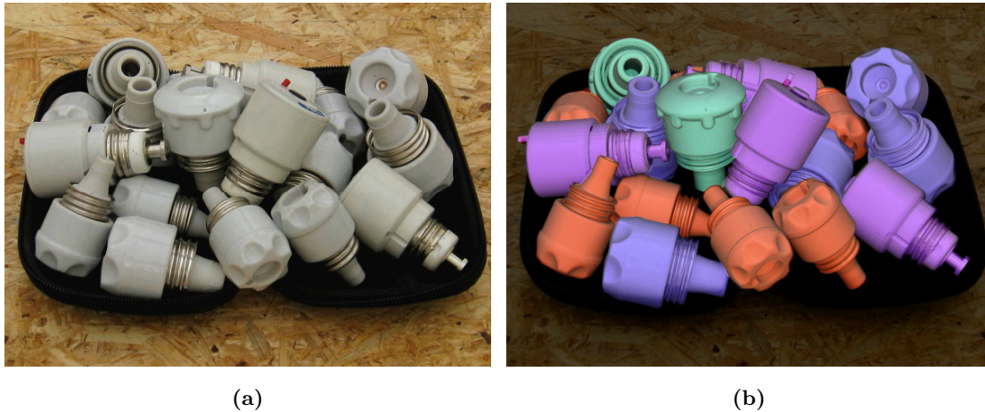
Figure 1.3: Shape-based 3D object detection and pose estimation using an RGBD camera. Shape-based approaches are particularly useful for detecting texture-less objects (a). CAD models of the detected objects are overlaid on the camera image (b). Images taken from the T-LESS dataset [1]. Copyright © 2017, IEEE.
