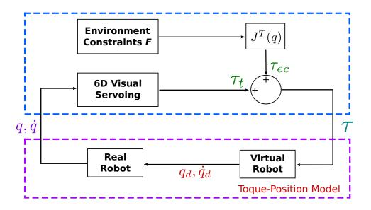
Figure 7.1: 6D visual servoing framework with environment constraints.
