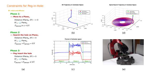
Figure 8.9: Peg-in-Hole assembly tasks: (a) Task constraints, (b) 3D trajectory in Cartesian space, (c) Force and force error in z axis, (d) Spiral search trajectory, (e) Real experiment.
