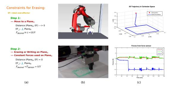
Figure 8.8: Erasing the board: (a) Task constraints, (b) Erasing task in simulation and real experiment, (c) 3D end-effector trajectory in Cartesian space and contact force from force sensor.
