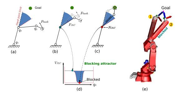
**Figure 8.2:** End-effector position control under joint limit constraints: In image (a), the robot's end-effector has been commanded to move toward a desired goal. The blue area defines a joint limit activation zone for the elbow joint. When this area is reached (b), a control approach is implemented to block the elbow joint while pursuing the goal (c). Image (d) depicts the attractor potential used to block the elbow joint inside the activation area. (e) shows the experiment results.
