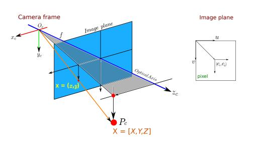
Figure 2.2: Pin hole camera model.
