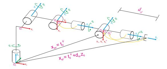
Figure 3.3: The StäubliTX90 configuration (6 DOF) for kinematic decoupling.
