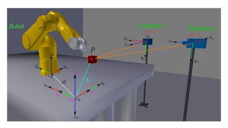
Figure 4.4: Geometric model of the orthogonal camera system.
