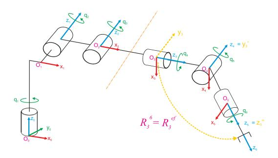
Figure 3.5: Spherical wrist: the final 3 joints of StäubliTX90.
