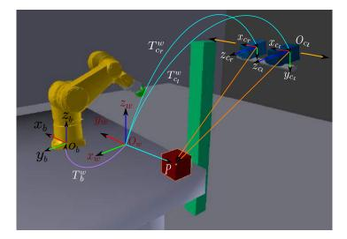
Figure 4.7: Geometric model of the stereo camera system.
