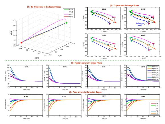
Figure 6.1: Simulation Test 1: Large translational and rotational motion.
