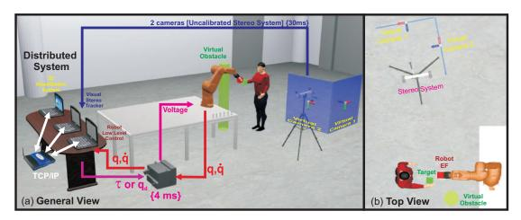
Figure 7.3: Robotic experimental setup in a Human-robot Interaction scenario.
