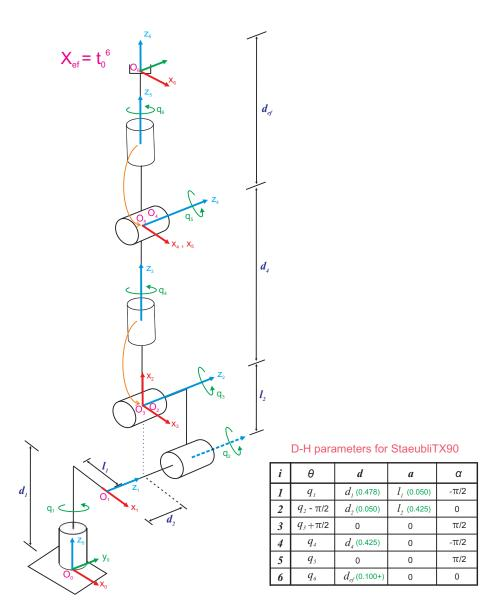
Figure 3.2: The StäubliTX90 configuration (6 DOF) and D-H parameters.
