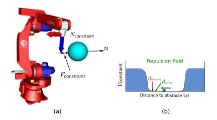
Figure 8.3: Obstacle avoidance: When an obstacle approaches the robot's body, a repulsion field is applied to the closest point on the robot's body.
