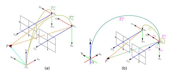
Figure 4.8: The stereo camera model: (a) shows a 3D point projected in two cameras, (b) the world coordinate frame is on the left camera frame point.
