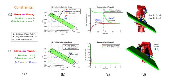
Figure 8.4: Motion constraints tests for robot manipulators in two cases: (1) Move to a plane; (2) move on a plane. (a) Constraints for tests, (b) 3D position in the task space, (c) control parameters, (d) 3D visualization of coach for simulations.
