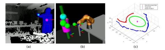
**Figure B.4:** Avoid Human: (a) Tracking human skeleton using Kinect; (b) Human joints model; (c) Human avoidance results: robot movement (red line) and target movement(blue line), Human position (green circle).
