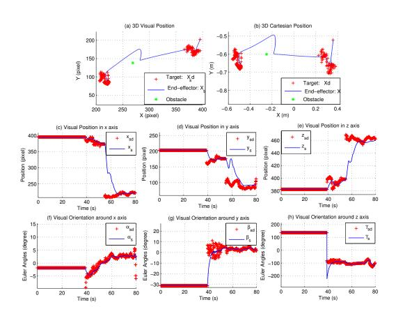
Figure 7.7: Position trajectories with obstacle avoidance.
