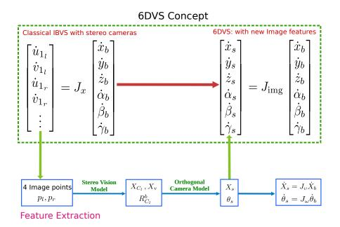
Figure 5.2: Algorithm design: mapping from the classical IBVS features to new orthogonal features in the virtual visual space.
