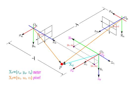
Figure 5.4: Placement of the virtual composite camera model with respect to left camera.
