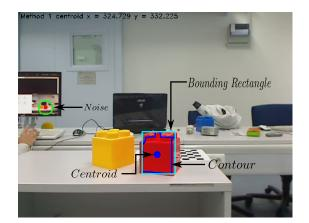
Figure A.2: The results of color-based objects detection.
