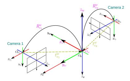
Figure 4.5: Two orthogonal camera configuration.
