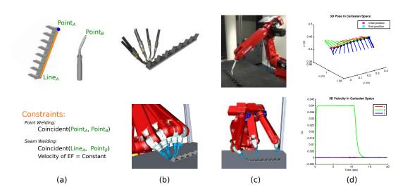
Figure 8.7: Welding in a robotic workcell: (a) Task constraints, (b) point welding, (c) seam welding in simulation and real experiment, (d) 3D end-effector trajectory and velocities for robot end-effector.
