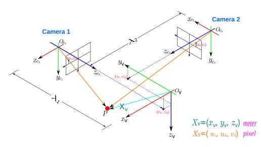
Figure 4.2: Two projective cameras which are orthogonal.
