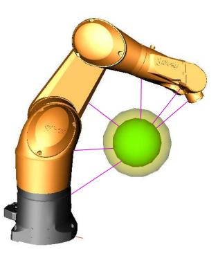
Figure 7.2: Computing the repelling forces of an obstacle.
