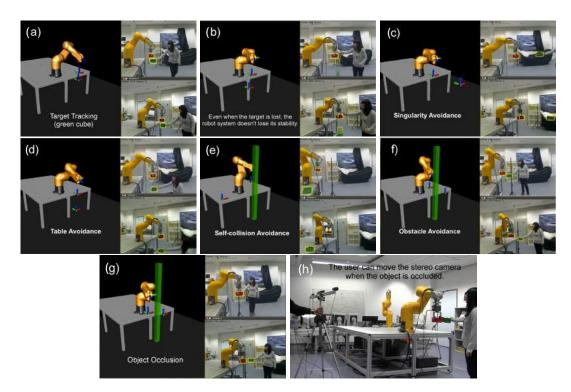
**Figure B.5:** System behaviors: (a) 3D Position tracking. (b) Case when the target is lost. (c) Case with singularity avoidance. (d) Table avoidance. (e) Self-collision avoidance. (f) Obstacle avoidance. (g) Case when the object is occluded. (h) The camera can be moved when the target is occluded.
