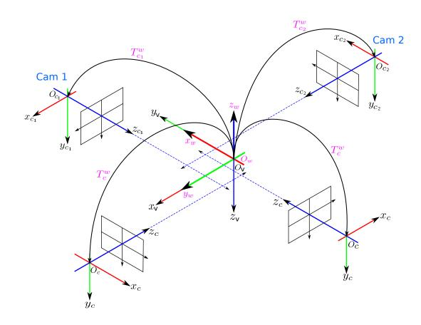
Figure 4.6: Four orthogonal camera configuration.
