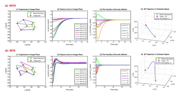
Figure 6.4: Simulation Test 3: Reaching (or not) a local minimum.
