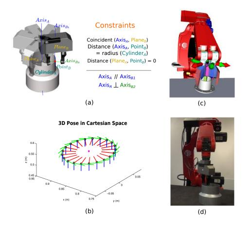
**Figure 8.6:** Grasping of cylindrical objects at their rim in a robotic workcell: (a) Task constraints. (b) 3D pose in Cartesian space, shows the end-effector trajectory. (c) and (d) illustrate the snapshots in simulation and real experiment.
