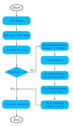
Figure A.1: Color-based objects tracking algorithm.
