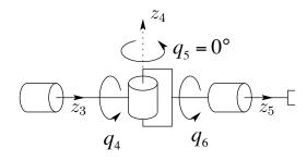
Figure 3.6: Spherical wrist singularity.
