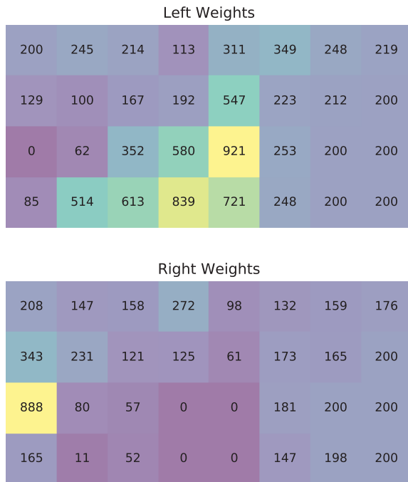
Fig. 10: Scenario 2. Learned connection weights to the left and right motor neuron of the R-STDP controller after 30000 simulation steps.
