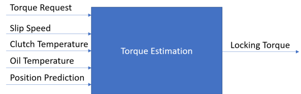
Figure 21: Actual transmitted torque estimation
