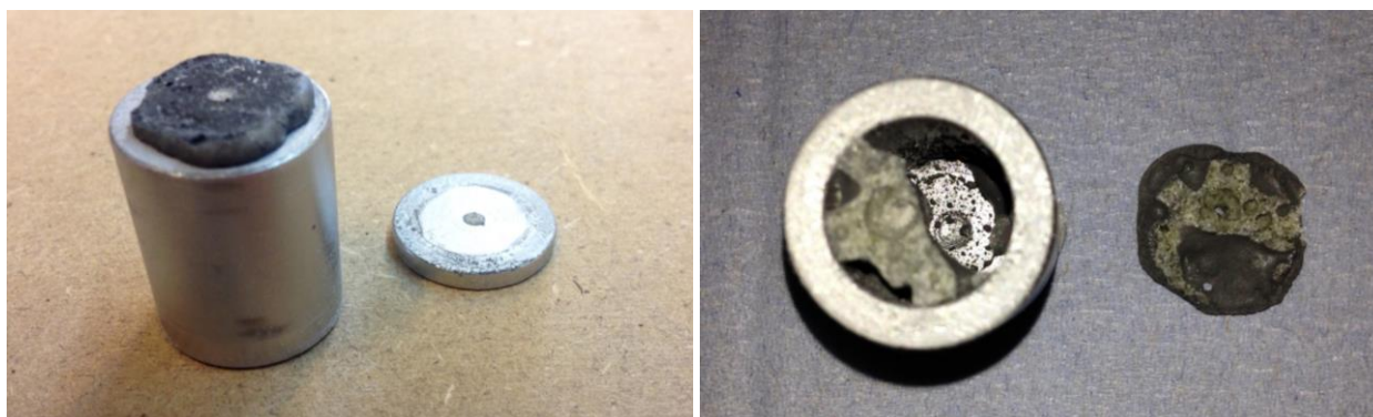
Figure 6-16: Oven after heating modes 3, 1, and 2, showing swollen and sintered sample with cavity (after breaking the sintered crust with a hammer)
