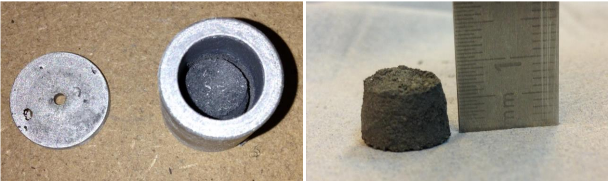
Figure 6-14: Oven after a number of preparatory tests, including heating up to 1180 °C, with significantly brighter surface and sintered regolith sample
