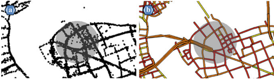
Fig. 4 Examples for selection areas in a global view with a FCD records as points and b classified road partitions
