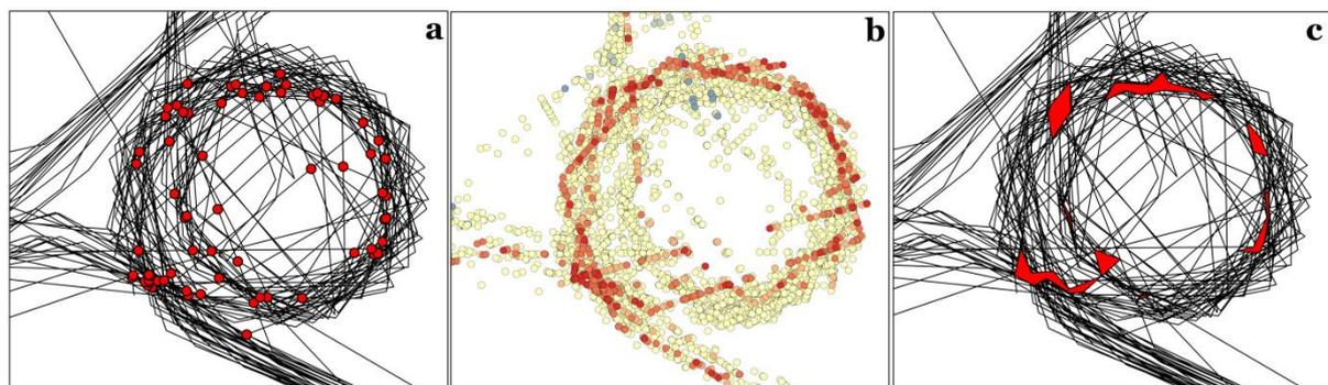
**Figure 2** Analysis of the taxi trajectories within the Nanpu on-ramp with (a) self-intersection points, (b) velocity hotspots from the Getis-Ord  $GI^*$  method and (c) distance-clustered self-intersections as convex hulls.
