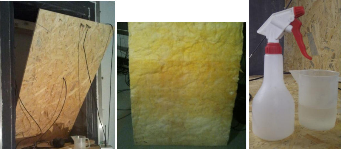
Figure 53. Sample after spray test with OSB panel (left), wet mineral wool (middle), spraying equipment
