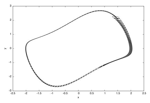
Figure 7.10: Plot of the van der Pol system (w = 0.2)
