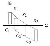
Figure 7.5: Iteration for computation of Poincaré map.
