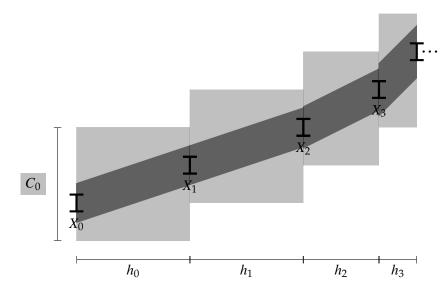
Figure 7.2: Illustration of rigorous one-step method.
