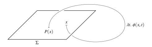
Figure 3.3: Illustration of Poincaré map *P* on Poincaré section  $\Sigma$ .
