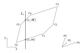
Figure 5.4: Corners and edges of a zonotope, intersecting line  $L_c$
