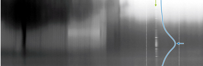
(b) Image of the VLC camera , showing the car boundaries projected from the detection camera image (a), and the signal pattern column produced by the headlight. The horizontal position of the column, and the vertical intensity profile (blue) are used to estimate the position of the sending headlight, to match it with the camera image in (a). Figure 8 shows the signal processing.
