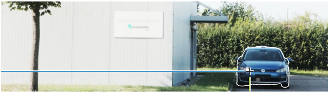
(a) Image of the detection camera , in which the sending car was identified using a convolutional neural network (CNN) trained for dynamic scene labeling (the “car” label is shown as a white outline); the active headlight position is extracted from the VLC camera image (b) (crosshair).
