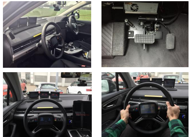
Fig. 1 Modified vehicle (RHDV) to simulate HAD. Top: steering wheel (left) and pedal dummies (right); Bottom: abstract take-over scenario (left) and steering impulse (right).
