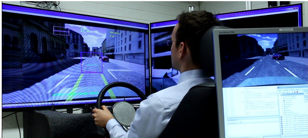
Figure 5.15 : A hazardous scenario while teleoperated driving with the time delay of 500 ms. The screen behind the operator shows the environment without time delay.
