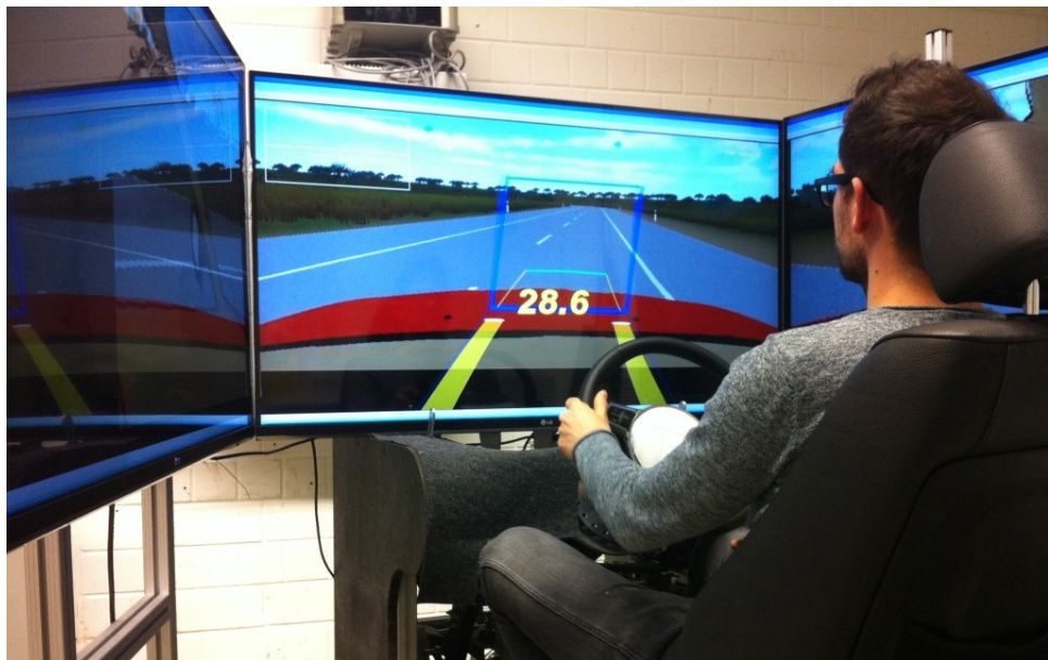
Figure 4.1 : A human operator controls the remote vehicle using the conventional operator's workstation.
