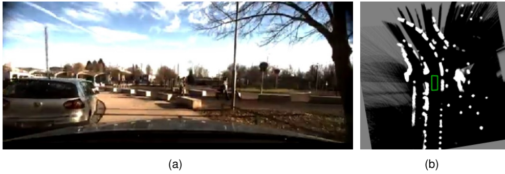
Figure 4.9 : (a) A narrow passage captured by the front camera of the remote car and (b) its corresponding 360° occupancy grid map created by two LiDAR sensors [144]
