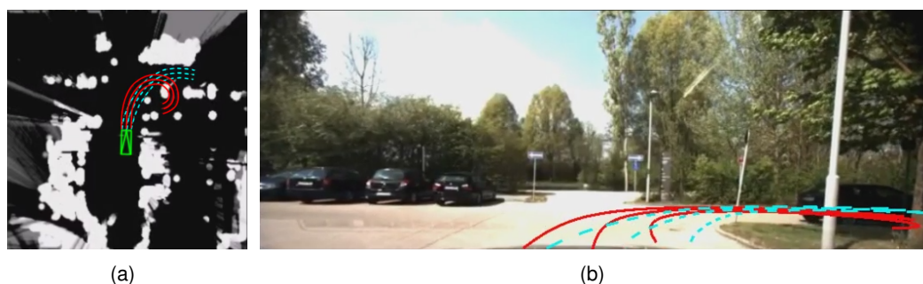
Figure 7.3 : Comparison of the manually generated path (red) as well as the autonomous generated path (aqua) [143]
