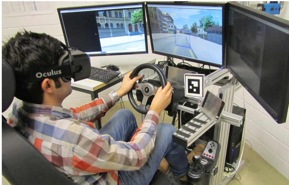
Figure 4.17 : The used operator's workstation for evaluation, equipped with three monitors and a head-mounted display to compare both visualization possibilities [144]
