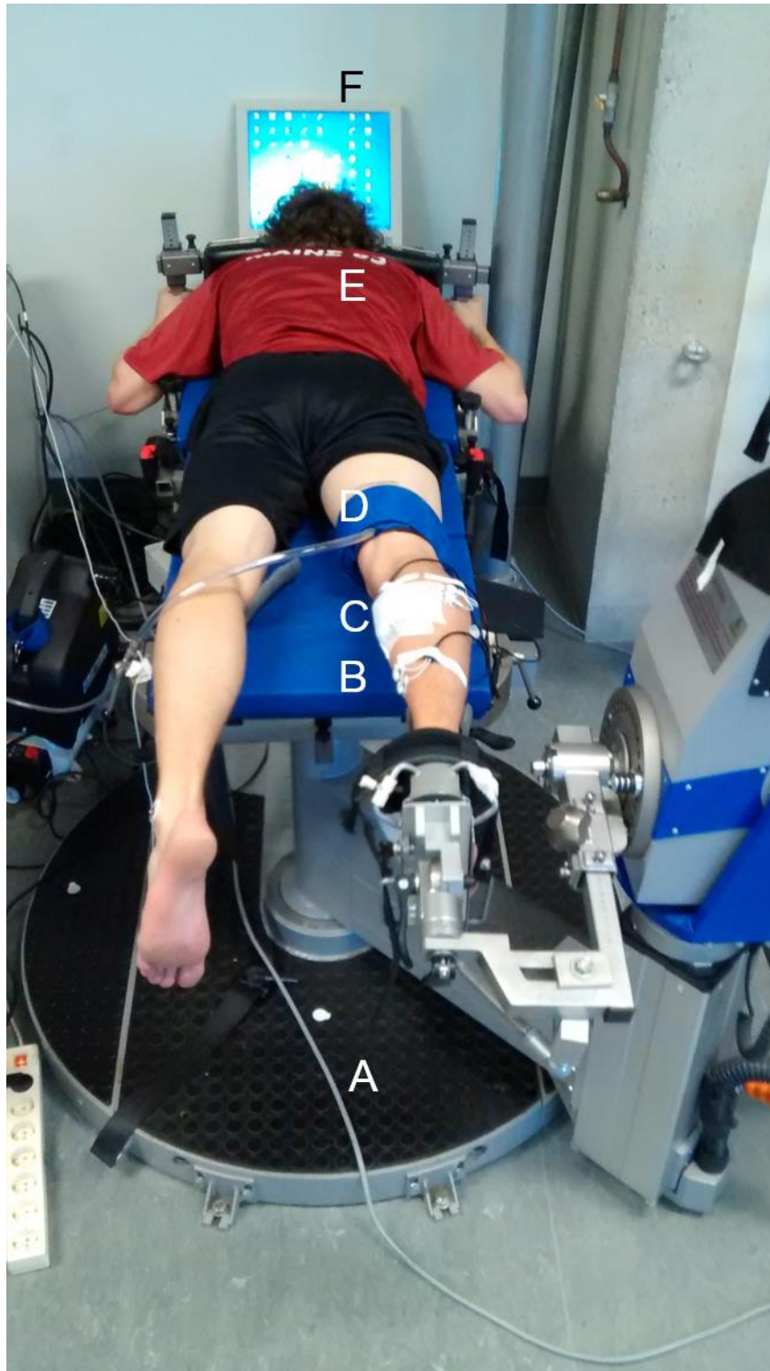
Figure 12: Experimental Setup: A) Motor-driven dynamometer. B) Electromyography system. C) Near-infrared spectroscopy device. D) High Pressure cuff. E) Shoulder pads. F) Screen for biofeedback
