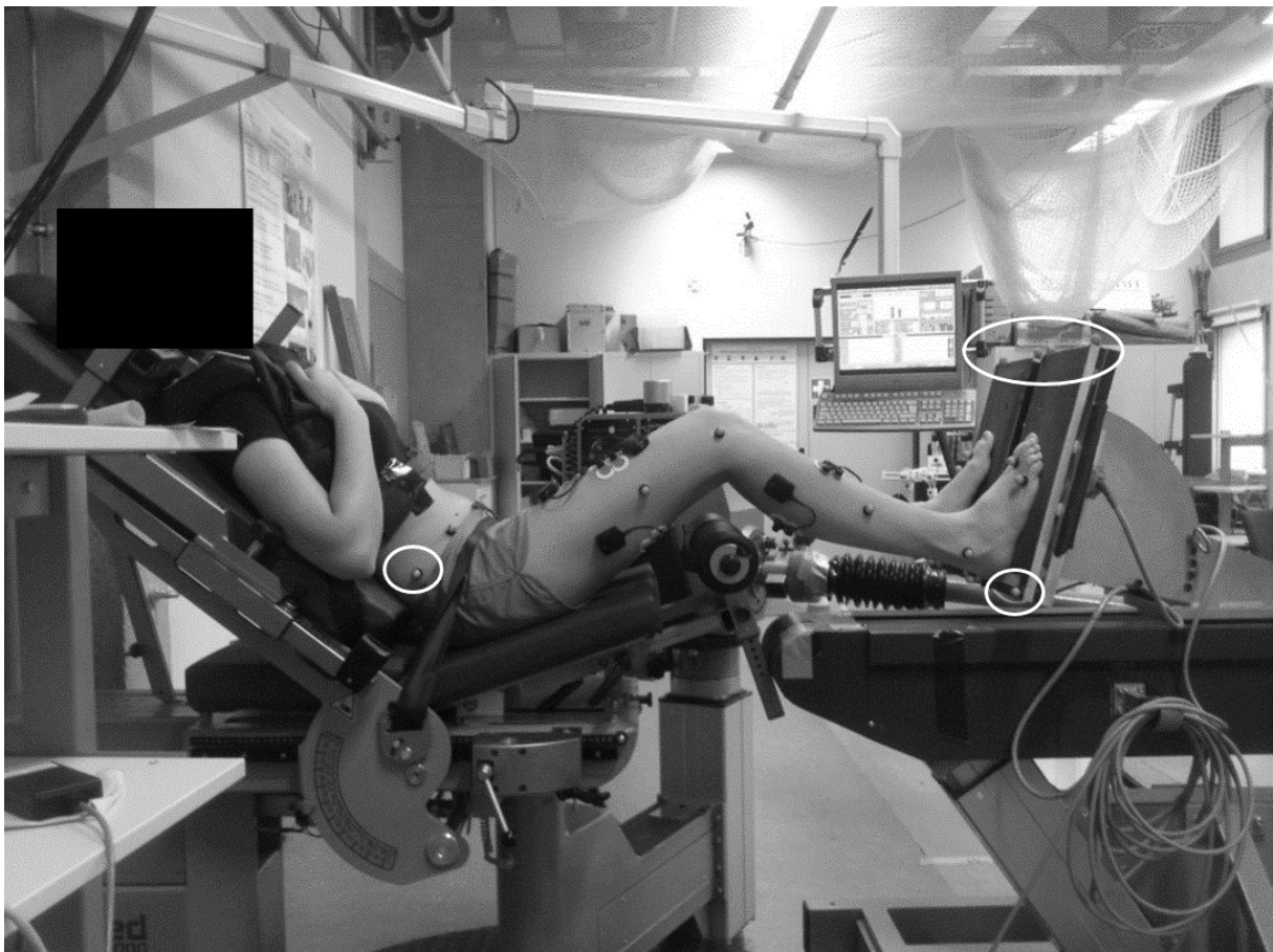
Figure 7: Example figure of a subject during a multi-joint leg extension setup, including force plates top mounted on the footrest of the leg-press adapter. Note: White circles show the adaption of the used marker set-up exemplarily.
